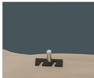
Figure 1. Template, UP marking up, spacer bar threaded in
