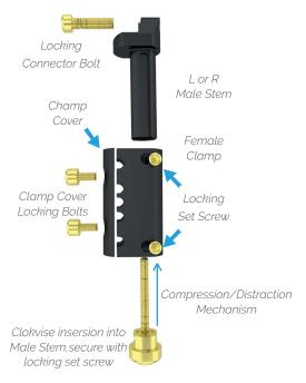
Modular compression/distraction mechanism provides incremental excursion (compression/distraction) capability to the telescoping fixator arm component. The modular C/D mechanism is turned clockwise into the threaded hole in the end of the male stem. It is then positioned such that the flat side of the mechanism faces the locking set screw. The locking set screw is then secured.
