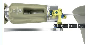
Loosen the wire locking bolt. Proper tensioning should commence from the side opposite to the olive.
