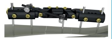
Supplemental fixation may be employed when off plane or additional single screw placement is required utilizing the supplemental bone screw clamp. A bone screw shank is secured to another bone screw shank within the proximal or distal bone screw cluster by means of a 6 mm connecting rod.
