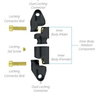
The inner body rotation component is comprised of two portions: inner body male and inner body female. When male and female portions are joined care should be taken to insure that serrated discs and locking set screw are in line. Assembly is then correct and set screw is tightened. This component allows 360° of rotation about the axis of the fixator.
